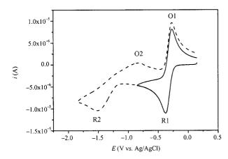
Figure 5. Cyclic voltammograms for the reduction of **8** (2 mm) in MeCN/Bu<sub>4</sub>NPF<sub>6</sub> (0.1 m) at v = 0.1 V s<sup>-1</sup> and with the direction of the voltage scan being reversed at -0.85 V (solid line) and -1.85 V (dashes), respectively.
