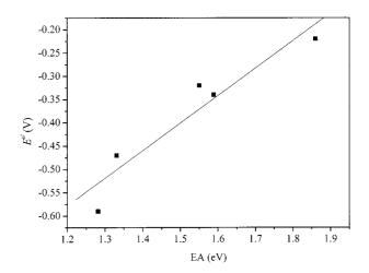
Figure 6. Plot of the  $E^{\circ}$  for one-electron reduction of the 1,4-benzoquinones (Table 2) as a function of the calculated electron affinities (EAs).
